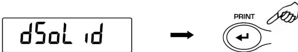
3. The density of the liquid to use will be displayed, the default value is equal to 1.0000 (distilled water at 20°C).
