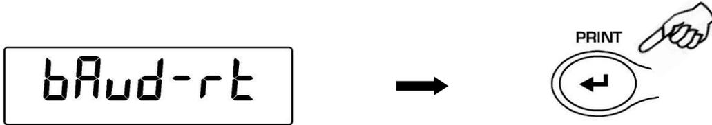
2. Select serial data transmission speed (1200-2400-4800-9600 baud). Pressing **MENU** or **CAL** buttons it will be possible to scroll forward or backward through the different transmission speeds, then confirm your choice by pressing **PRINT** button.
