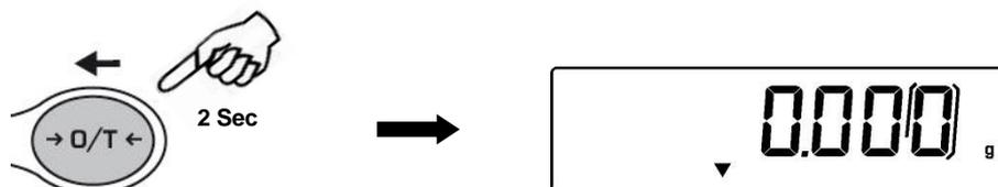
3. Insert now the desired tare value using the keys **CAL** and **MENU** for increase or decrease the value, and press the **O/T** key for skip to the following digit. During the value insert mode, if keep pressed the **O/T** key is possible to delete the inserted value.
