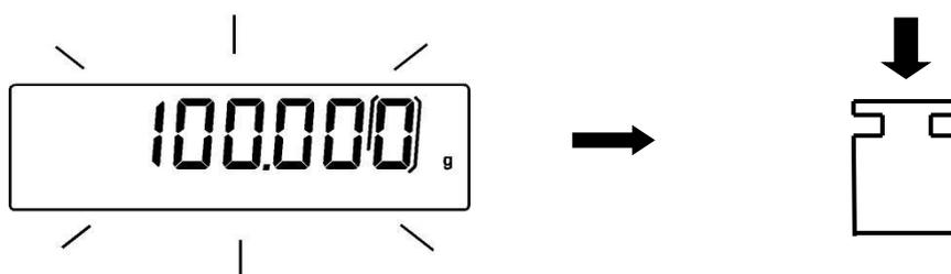
3. The display will stop flashing, indicating calibration weight value.
