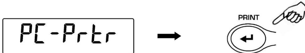
2. Press the **MENU** button until the “PC cont” is displayed to choose continuous print or “PC CMd” to choose print to PC at user command, then press the **PRINT** button to confirm the choice.
