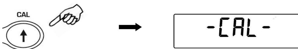
2. When calibration weight value starts to flash, load the weight on the pan.
