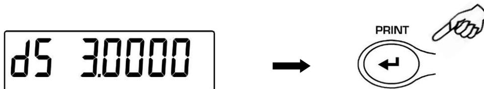
4. It is possible to set a different value using the **CAL** e **MENU** buttons for increase and decrease the value and using the **O/T** button for skip to the others digits. Keeping pressed the **O/T** button is possible to delete the inserted value.
