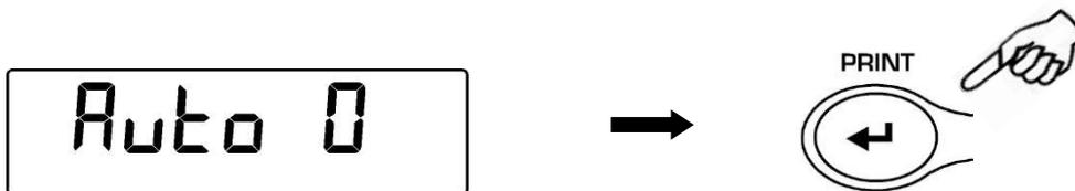
2. Pressing **MENU** or **CAL** button it will be possible to scroll forward or backward through the different autozero levels, select the one you wish and confirm it by pressing the **PRINT** button.
