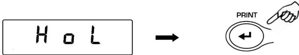
2. Insert the lower threshold value using the **CAL** e **MENU** buttons for increase and decrease the value and using the **O/T** button for skip to the others digits. Keeping pressed the **O/T** button is possible to delete the inserted value. The inserted value will be stored in the memory until the balance is switched off.
