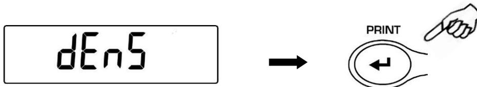
2. Using the **MENU** button, select the function “d Liquid” and confirm this with **PRINT**
