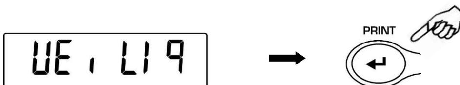
10. The result of the density of the liquid is now displayed. Pressing the **PRINT** button it is possible to print the value of density, if the balance is equipped with a printer.
