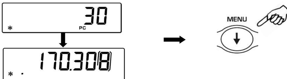
2. In order to display the weight of single piece from the total number of pieces press and keep pressed the **MENU** button until the acoustic alarm is over.
