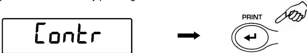
2. Now, pressing the buttons **MENU** or **CAL** it is possible to increment or decrement the level of the display contrast; select the one desired and confirm by pressing the **PRINT** button.
