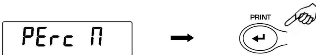
3. It is possible to set a different value using the **CAL** e **MENU** buttons for increase and decrease the value and using the **O/T** button for skip to the others digits. Keeping pressed the **O/T** button is possible to delete the inserted value. The inserted value will be stored in the memory until the balance is switched off.
