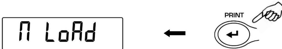
2. Activation of this function is indicated by the visualization of the letter **M** on the last digit on the display.
