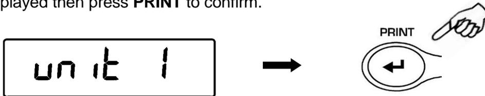
2. It will be displayed "**GRAM**" unit. Pressing the **MENU** or **CAL** button, it will be possible to scroll forward or backward the weight units menu.
