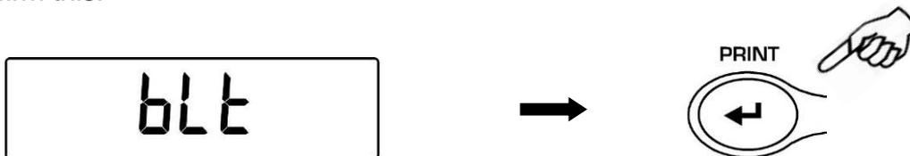
2. Pressing **MENU** or **CAL** button it will be possible to scroll forward or backward the different working modes, select the one you wish and then confirm it by pressing the **PRINT** button
