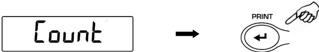
2. Select the number of pieces to put on the pan as sample by pressing **MENU** repeatedly to increase and **CAL** to decrease the number. Choice of the number of pieces (10, 25, 50, 100) depends from the weight of single pieces. If available, load the empty container first then press **PRINT** to confirm.
