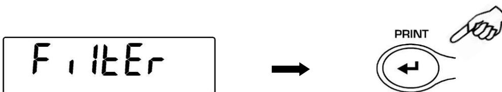
2. Pressing **MENU** or **CAL** button it will be possible to scroll forward or backward the different filtering levels, select the one you wish and then confirm it by pressing the **PRINT** button
