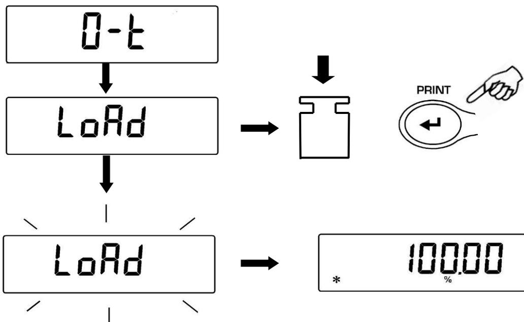
4. Remove now the reference weight and load the sample. Is possible to read the weight in percentage now.
