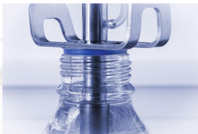
Figure 3: Best accuracy is reached if the metal tube is well immersed in the sample during the measurement due to best temperature equilibration
