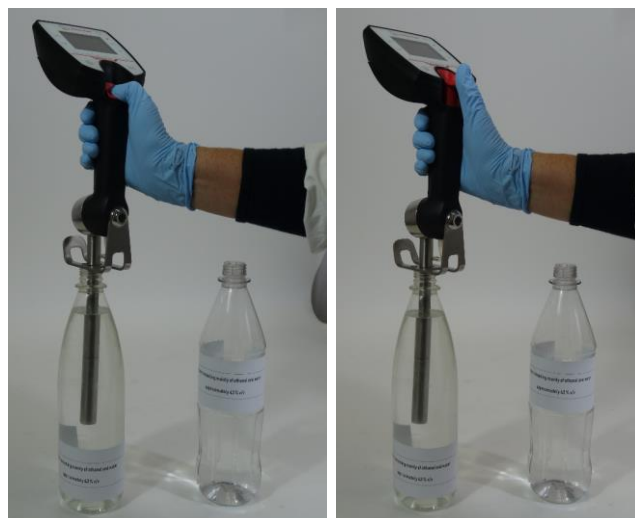
Figure 1: Immerse Snap 41 and release the pump lever
