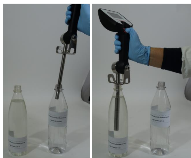
Figure 2: Discard the first 2 fillings, fill again, discard and fill while the instrument remains on the sample vessel
