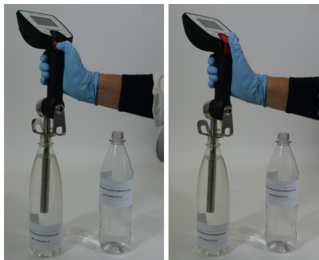
Figure 1: Immerse Snap 41 and release the pump lever
