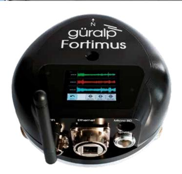
Ideal for earthquake early warning and structural health monitoring, the digital Fortimus accelerometer delivers ultra-low-latency strong motion data direct to your network.
